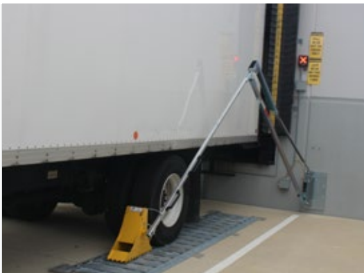
Two sensors—one on the unit and one on the wall—indicate when the unit is properly stored to prevent accidental damage.
