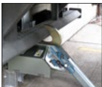
The TPR hook rotates up to engage and secure the trailer to the loading dock.
