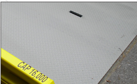
A 60" transition at grade and 30" transition at dock height is constructed of high strength diamond tread plate beveled and recessed for smooth transition onto and off the yard ramp.
